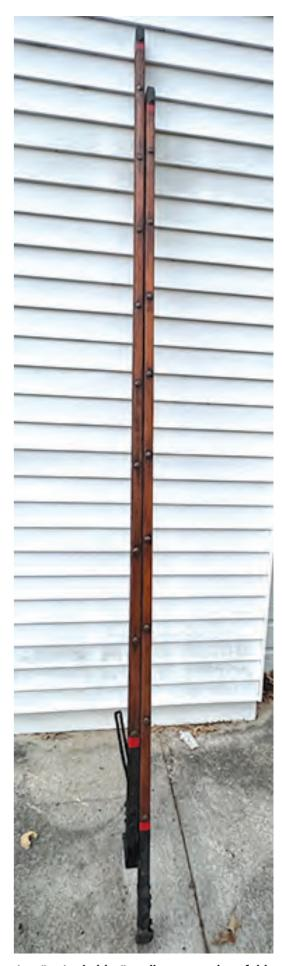
An "attic ladder" collapses and unfolds into a regular ladder. It's small size allowed firefighters to carry it into small places. They are still used, but made of aluminum, not wood like this one. Photo by Tom Chillemi
