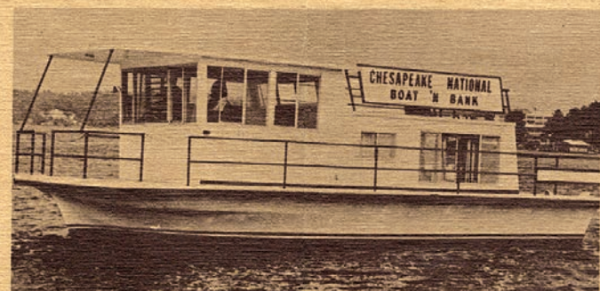
Chesapeake National's new "Boat 'n Bank" office is housed on a fiberglass houseboat. The craft is 33 feet long, weighs about 8,500 pounds and can reach a top speed of 30 mph.
