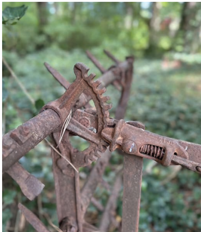
A harrow was used to smooth soil. The angle of the spokes was adjusted with a gear and lever.
