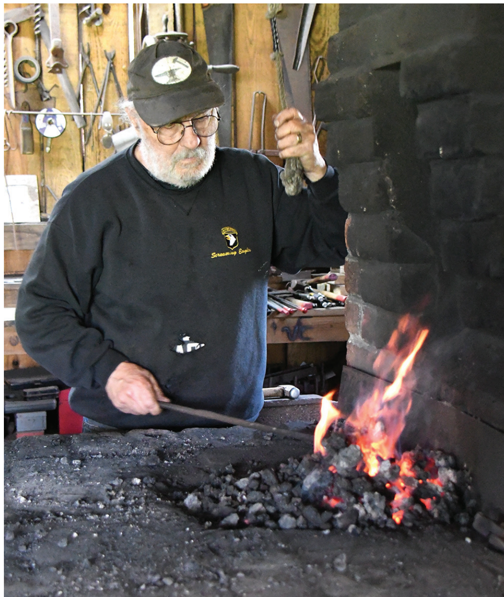
Ken Kauffman pulls a robe connected to the bellows which increases the airflow to the coals and intensifies the heat.
