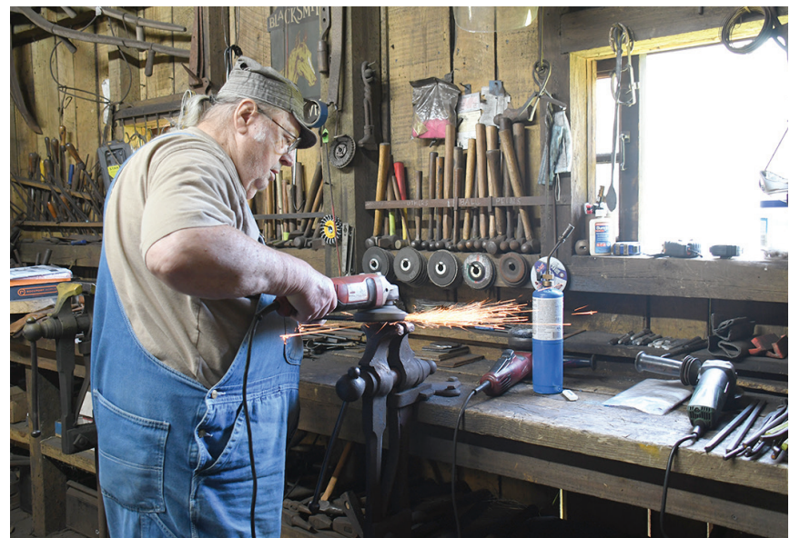
Instructor Roger Amidon uses an angle grinder to shine a piece of steel.
