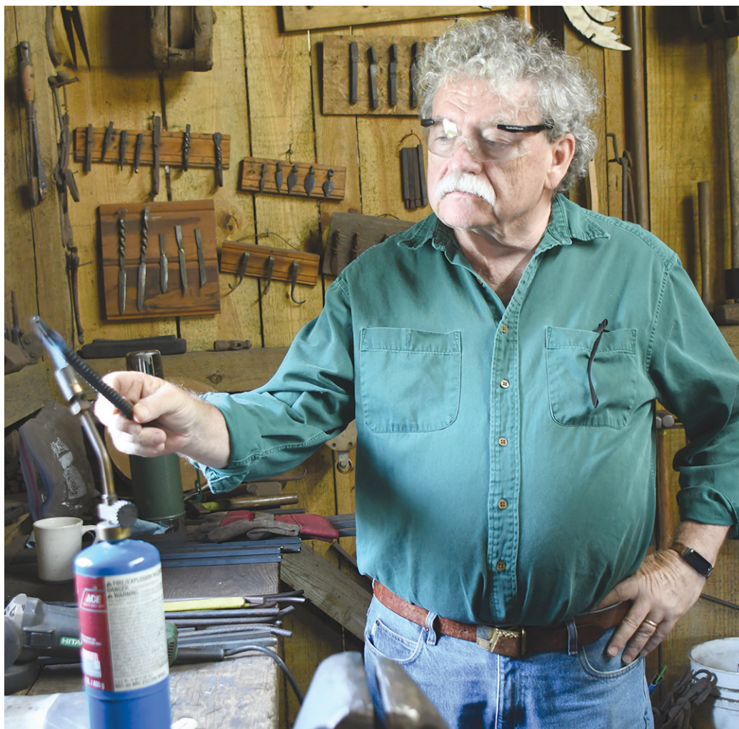
Frank Reilly heats a piece of iron over a torch. The iron is formed into a punch.
