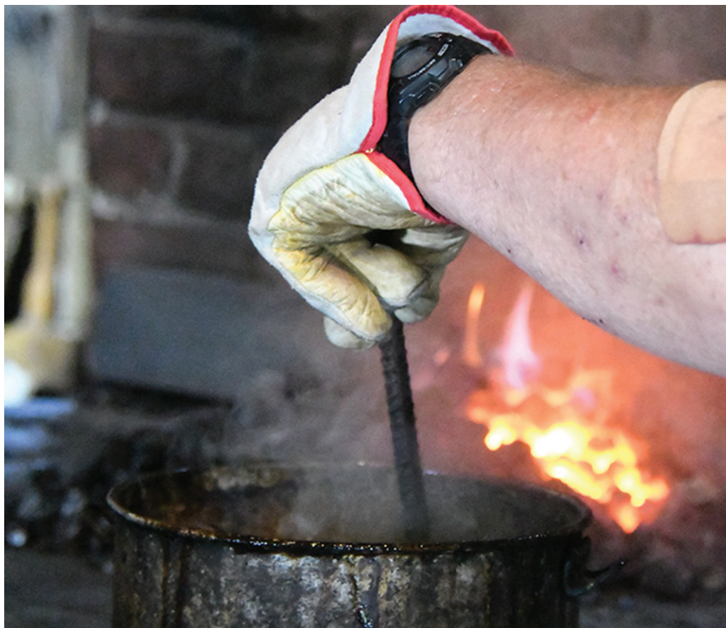
A hot piece of iron smolders as it's dipped into the cooling bath.
