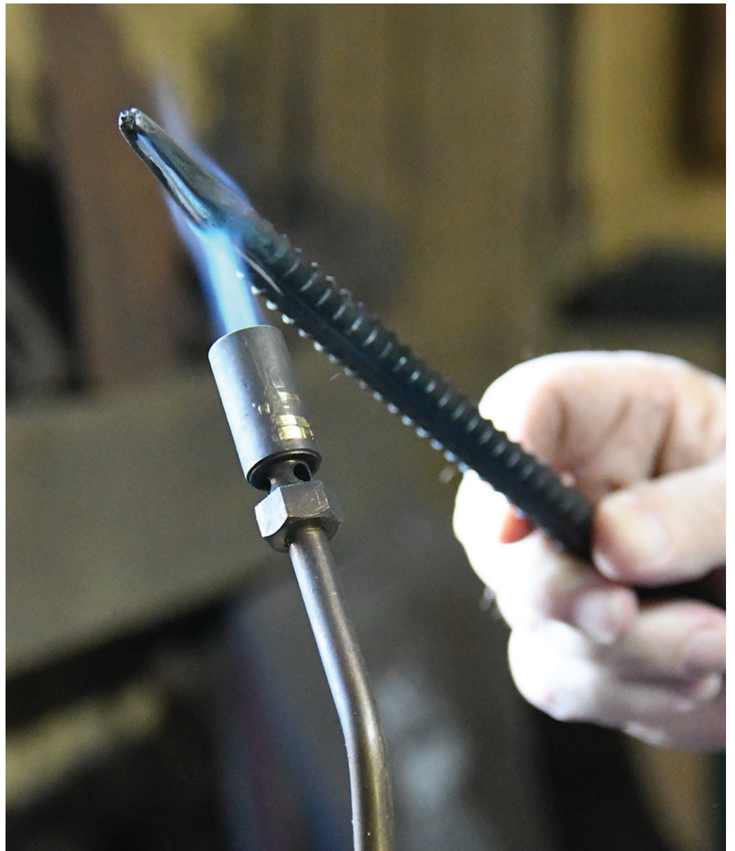
A torch is a controllable source of heat versus the fire, which allows for more precise temperature control.
